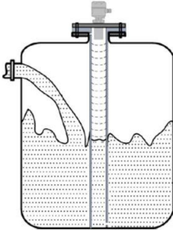
6.2.8 When install to the cold area, should choose the lengthen sensor of the level meter ,make the sensor extend into the container, shun frost and icing.
