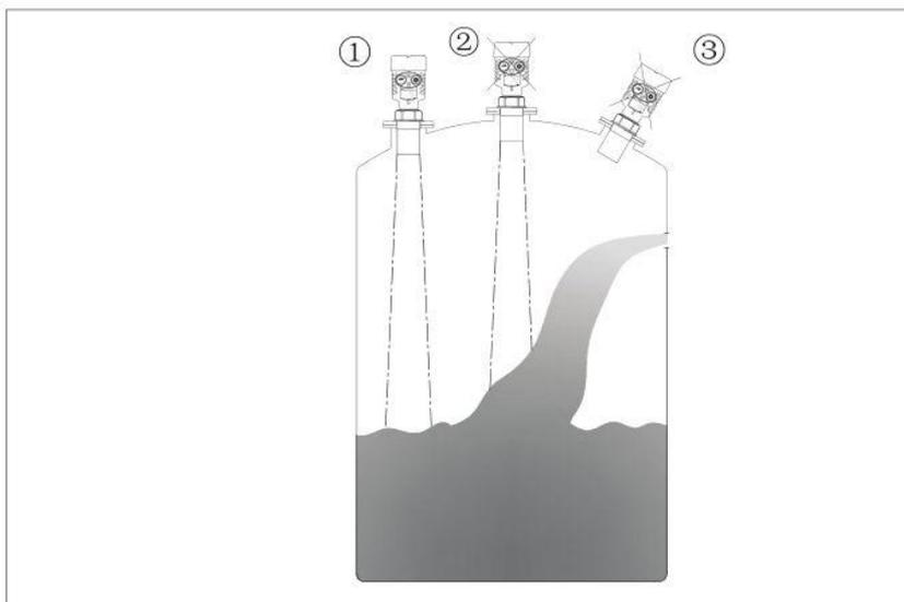
6.2.3 Meter Installation should be avoid A.B obstacle
