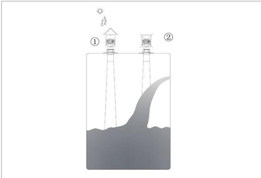
6.2.2 Energy transducer should be vertical to the measuring medium surface
