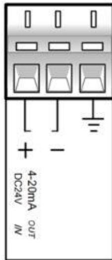
Note: Power supply for DC24V level meter itself, Please pay attention to the wiring signs. Outer loop should be have current power supply capability of 30mA.
