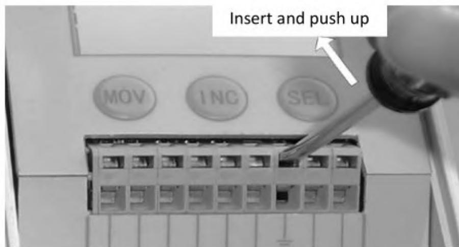
The terminal blocks are all self-tightening ones. Use a straight screwdriver to wire as follow. Please noted the the power supply specification and polarity. Outer ring circuit should with 30mA current power supply capability.
